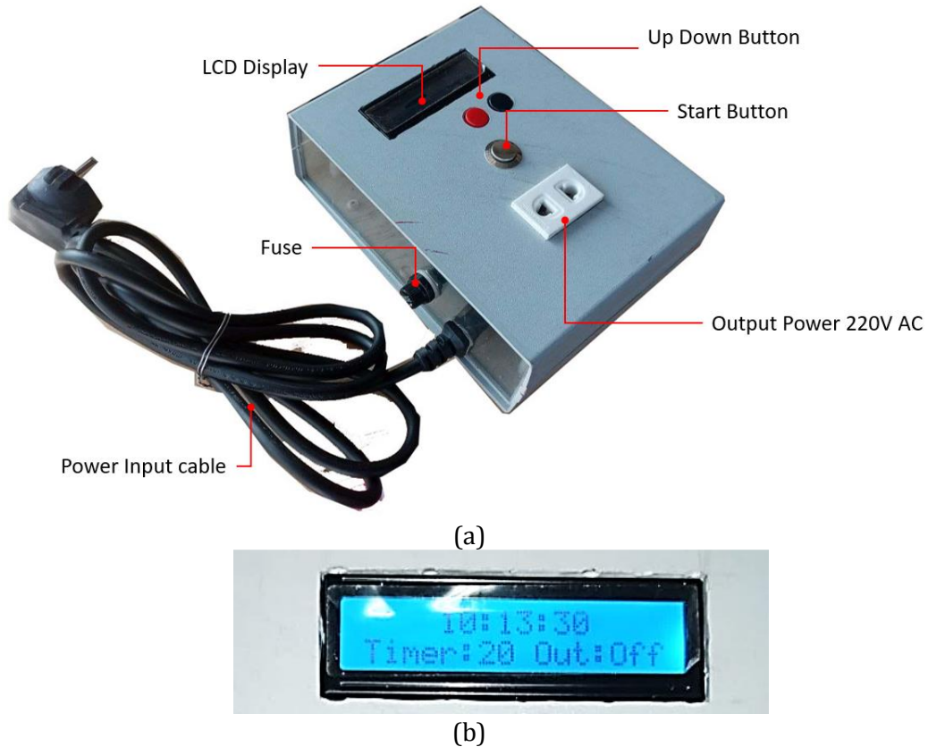
Figure 6. Display the device, (a) name of each part of the device, (b) Display of LCD, hour timer and status of output
