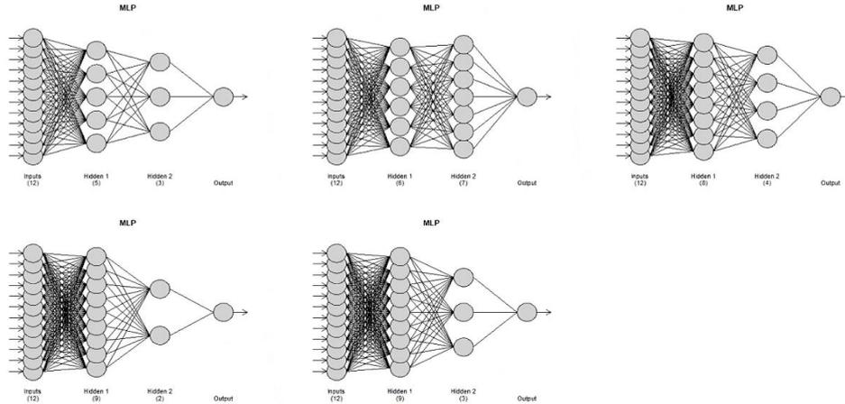
**Figure 4.** Architecture of MLP Models
