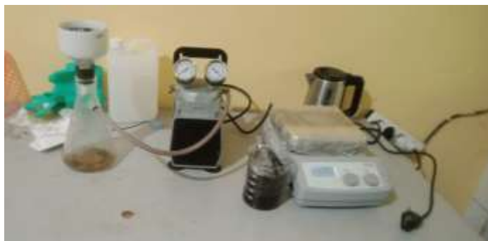
Figure 2. Extraction Process SiO 2 from Water Hyacinth.
