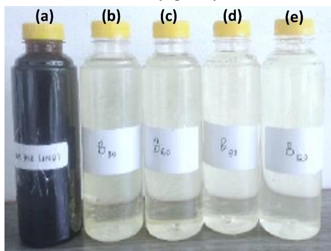
Figure 2. Leachate samples before and after processing using the Fenton method at various time variations (a) 0 min, (b) 30 min, (c) 60 min, (d) 90 min, and (e) 120 min
