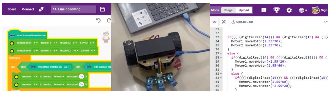
Figure 5. Block-based code sequence transferred to hardware
