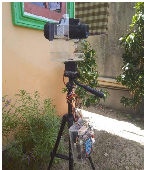
Figure 16: Arduino-based Rukyatul Hilal instrument seen from the side.
