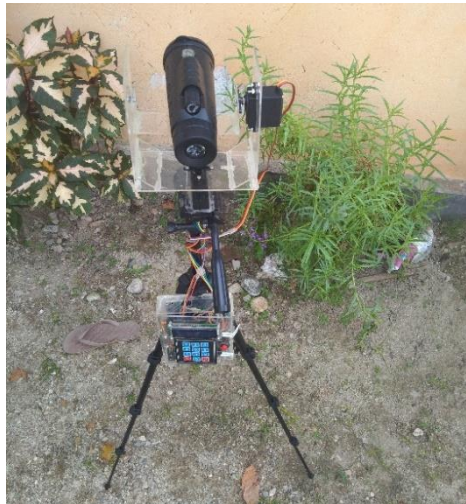
Figure 15: Arduino-based Rukyatul Hilal instrument seen from above.
