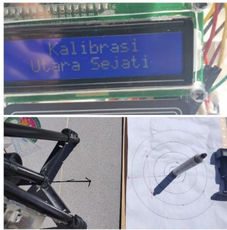
Figure 17: The results of the northern comparison of the Arduino-based Rukyatul Hilal Instrument and the Sun's shadow method using a special stick
