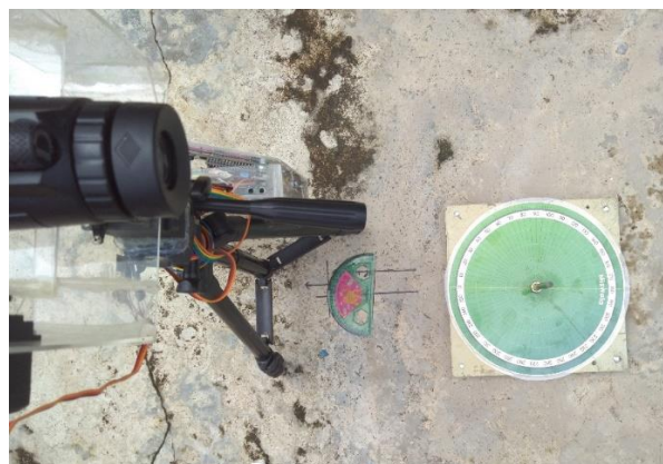
Figure 18: Comparison of true north measurements using Mizwala and Arduino-based Rukyatul Hilal Instruments
