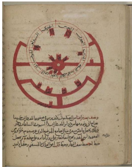
Figure 2. The rete ( ankabūt ) in al-Farghānī's manuscript showing stellar positions and the ecliptic circle.
