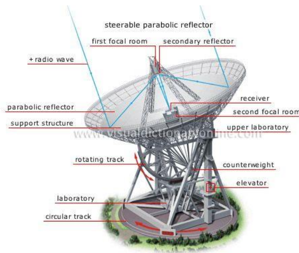
Figure 4. Radio Telescope Components
