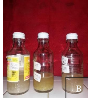
Figure 1. Color changes in the media exhibited by the bacterial isolates at 28°C after 14 days of incubation (A: High-Density Polyethylene Plastic; B: Low-Density Polyethylene Plastic)
