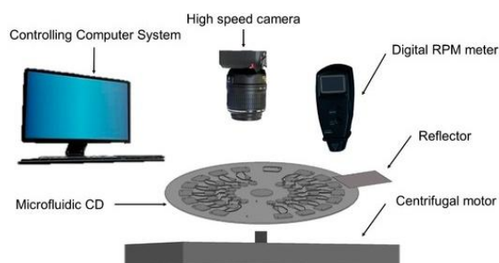
Figure 4. The complete experimental setup includes a computer-controlled system and a custom Lab-on-a-Disc (LoD) spinning test system. Reproduced from Abd Rahman et al. (2018), published by Multidisciplinary Digital Publishing Institute, licensed under CC BY.
