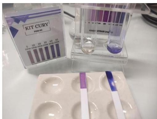
Figure 4. Comparison of mercury ion detection between the developed strip test and the commercial kit
