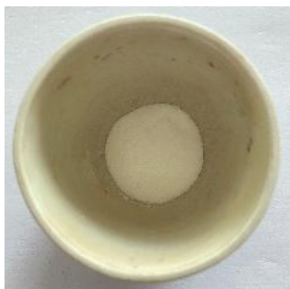
Figure 5. White dried silica aerogel
