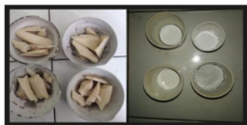
Figure 4. Before (left) and after (right) calcination of beef bones at 900°C.
