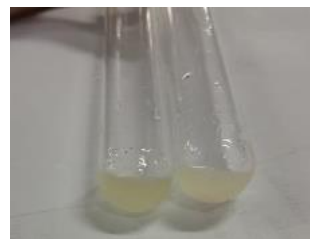
Figure 6. FFA qualitative test results (right: corn oil, left: palm oil)
