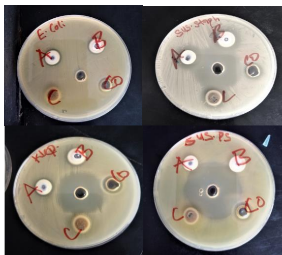
Figure 7 : Antibacterial activities of JC-ZnO NPs in the petri dish: E. coli (A), S. aureus (B), K. pneumonia (C), P. aeruginosa (D)
